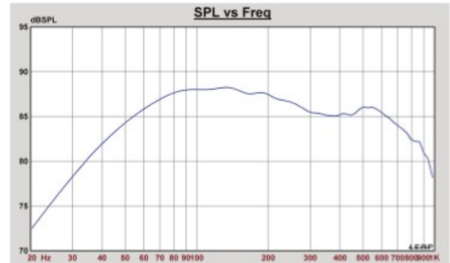
The graph above shows the measured sound pressure level on axis (0 degrees) in the low frequency (20 - 500Hz), using a 30Ltr sealed box. Response is measured in near field, and normalized to 1m, 2π radiation, 1/12 octave smoothing is applied. Input voltage is 2.83V RMS. Sensitivity is calculated at 100Hz on axis.
